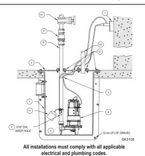
TYPICAL FLOAT HANGER ON STEEL COVER PITS
